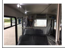
Passenger clear vinyl guards easily pull down and latch to make it easy for your passengers to protect themselves. The clear guard does not impede passenger viewing or fully restrict air flow.
